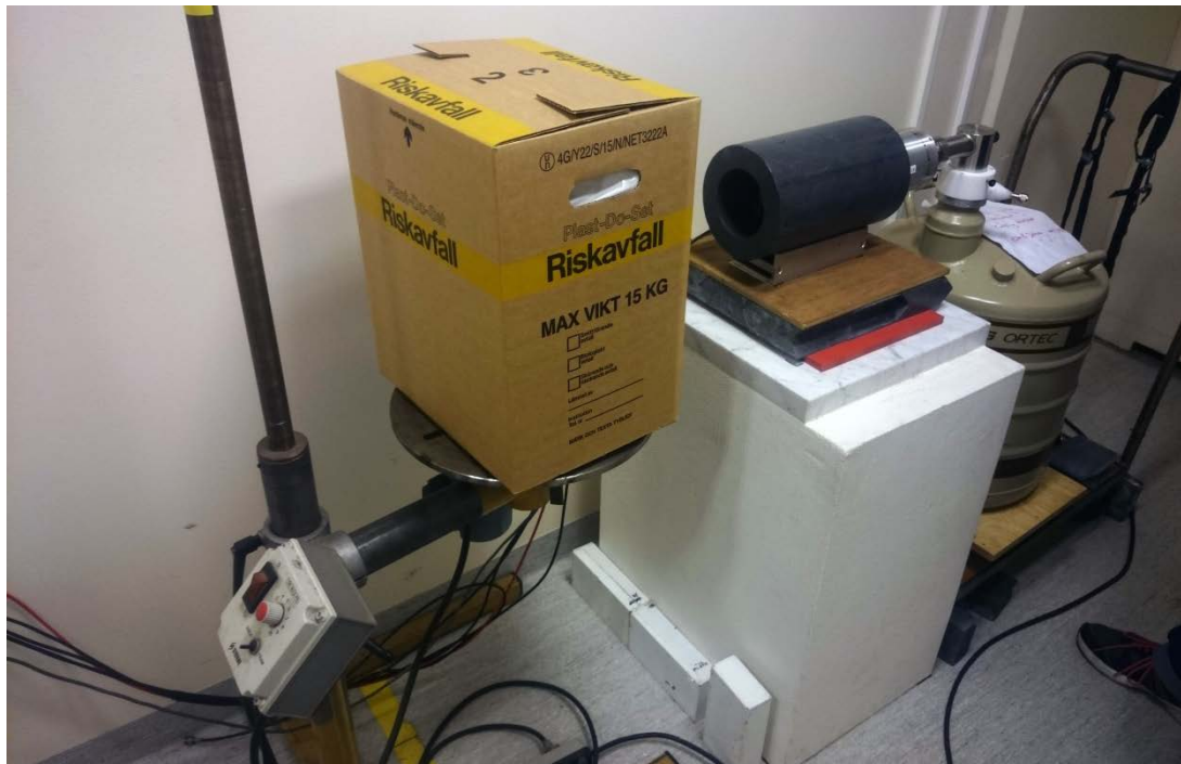
Picture: Waste box on a turn table on the right, in front of the HPGe detector on the left
